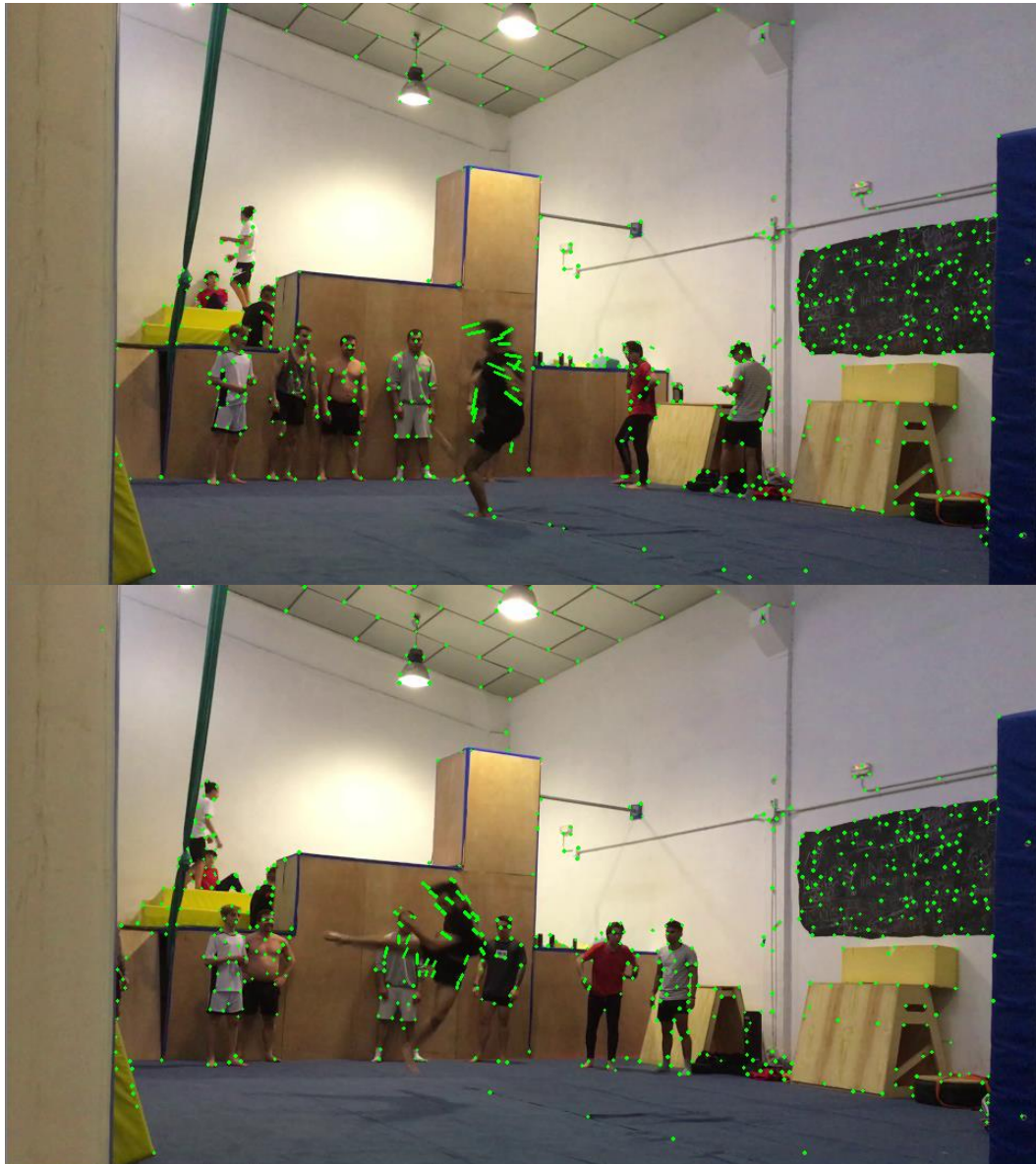
Figure 9. Example of the motions estimated using a pyramidal implementation of Lucas-Kanade algorithm for two different frames.
